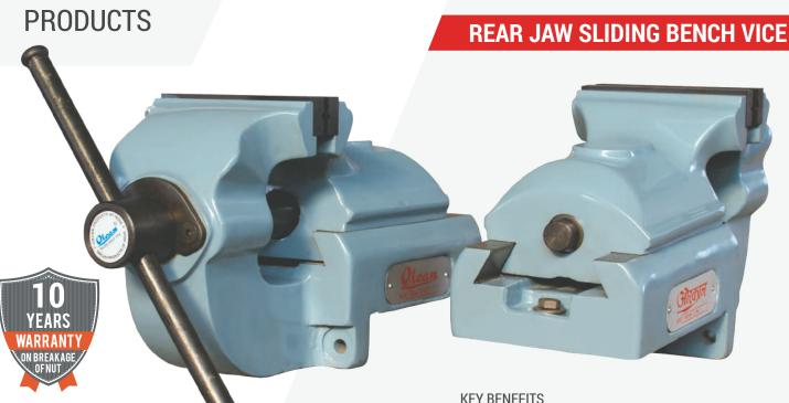
Unique rear jaw movement design eliminates breakage in front jaw, saves valuable space towards operator as front jaw is stationery. Right angle machined mounting surfaces with two hole in front and one at back eliminates shaking and swivelling of vice.
